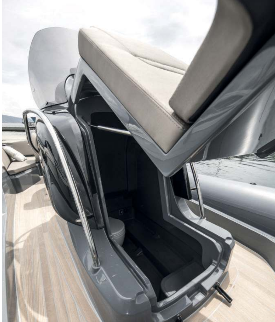
Toilet under console
