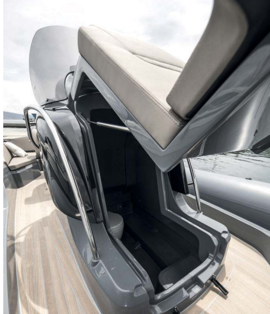
Toilet under console
